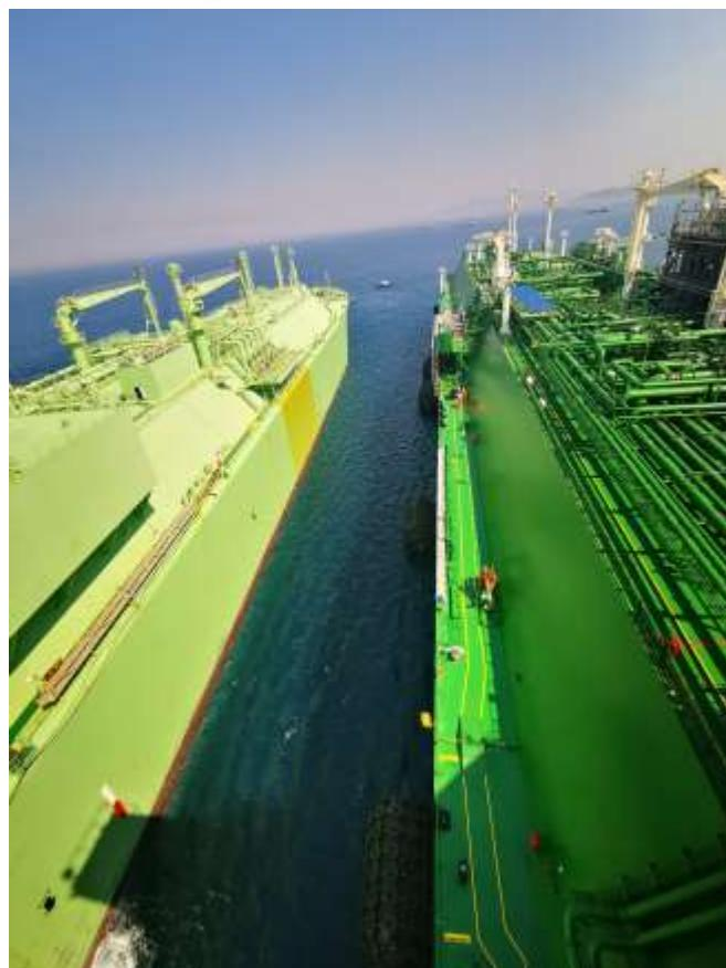
The LNG vessels range up to Q-Flex size shall be moored, unless a different mooring arrangement is submitted to and approved by the FSRU Operator and Terminal Management in advance. It shall be noted that a ship specific SSCS (Ship to Ship Compatibility Study) shall be performed and / or verified by the FSRU Operator for each vessel visiting the FSRU and Terminal.
