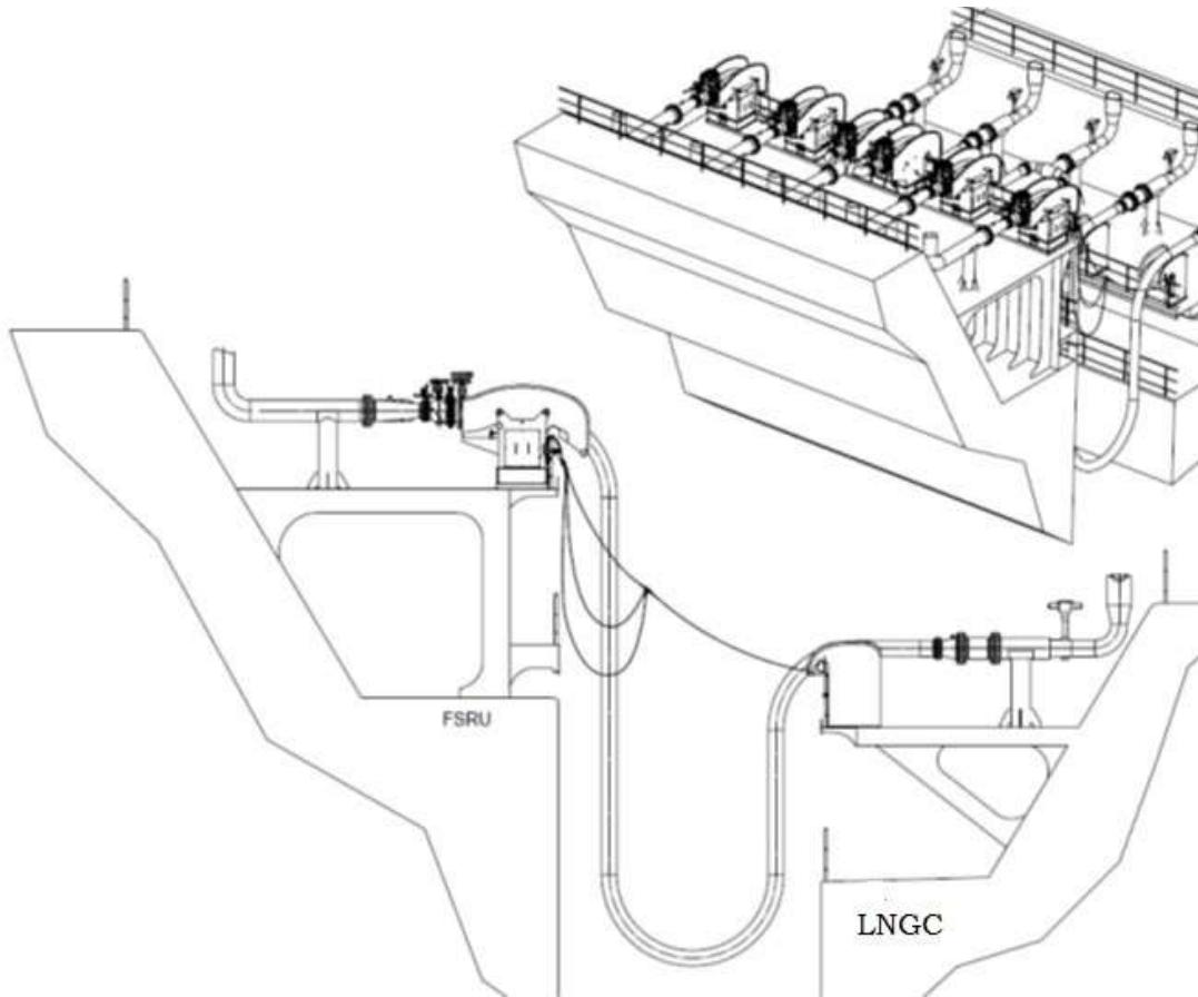
When the cargo transfer hoses are stowed on the FSRU when not in use, the hoses shall be stowed and maintained under a slight positive-pressure nitrogen and ambient temperature.
